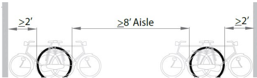
Figure 4: Spacing Requirements for Racks Installed Perpendicular to an Aisle in the Middle (credit: SFMTA)
